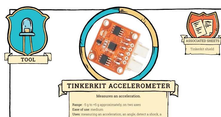
This sensor measures the acceleration in two directions, X and Y, represented on the sensor. The acceleration in the third direction, Z, is not available. This sensor requires two cables for the connection, one for each direction.
