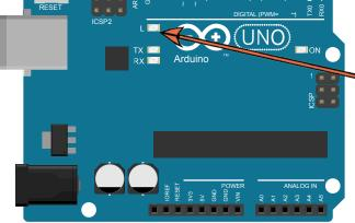
Small test light-emitting diode (LED). This LED is connected to digital port 13 on the majority of Arduino boards.
