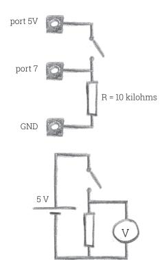
When the switch is open, port 7 and the ground are connected and are at the same electrical potential because no current is circulating: the board measures 0 V (LOW). When the switch is closed, the potential of the input 7 rises to 5 V (HIGH) and a current of 0.5 mA is circulating between the 5V port and the GND port, which poses no problem.
