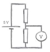
The setup above allows you to measure a voltage modified by a potentiometer comprised of between zero and five volts. This setup is equivalent to a voltage divider (see the equivalent diagram).
