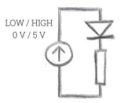
To control a LED, the uploaded program on the microcontroller must define the digital port 2 as output (see Challenge sheet "Light up a LED").
