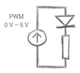
If one needs a real continuous analog voltage, one must install a low-pass filter that will eliminate the high frequencies and only keep the average value (the frequency of oscillation of the PWM output is around 500 to 1000 Hz depending on the ports).
