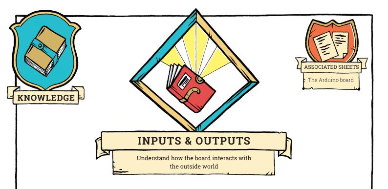
The input/output (I/O – input/output) represents the way in which the Arduino board interacts with the outside world. The outputs are controlled by the board allowing the microcontroller program to trigger actions (switch on or switch off a LED, a ventilator or a motor). The inputs are read by the microcontroller which allows it to become aware of the state of the system that it is linked to.
