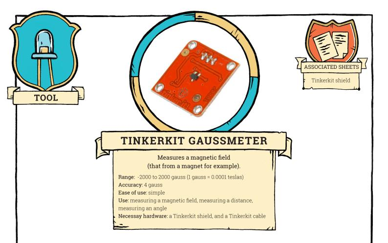
This sensor uses a Hall probe to measure the magnetic field.
