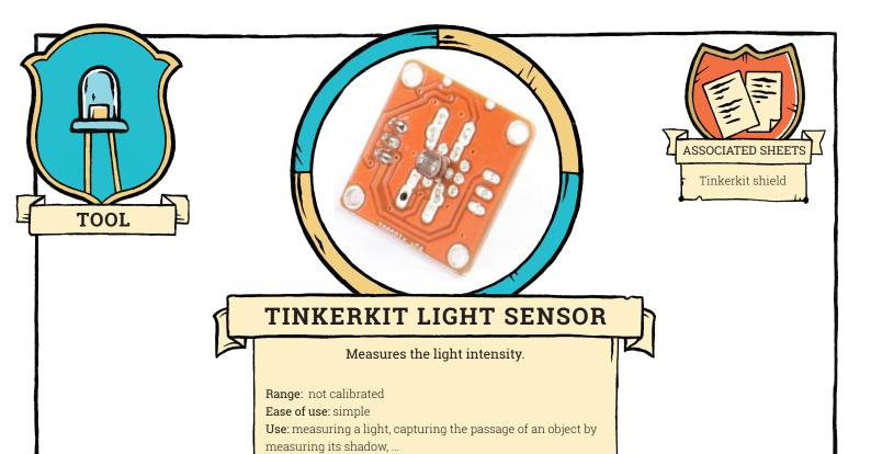
This sensor uses a resistance whose value varies with illumination (Light Dependent Resistor) to measure the light intensity that illuminates the sensor.
