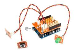
For the Uno version, the shield offers 6 inputs, white connectors, labelled IO, II, ..., I5, and 6 outputs, orange connectors, labelled OO, OI, ..., O5.
