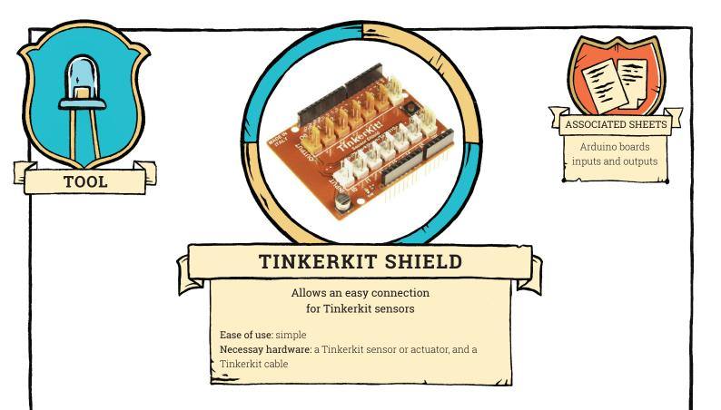
The term "Tinkerkit" includes a family of sensors and actuators that can be easily wired to an Arduino board with special cables and a suitable shield. The cables include three wires, a ground wire (black), a 5-volt power wire (red), and a data wire (orange).
